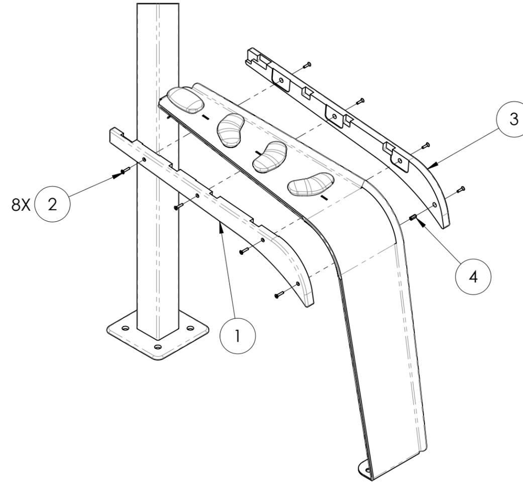
ASSEMBLE SIDE PANELS WITH ITS HARDWARE
